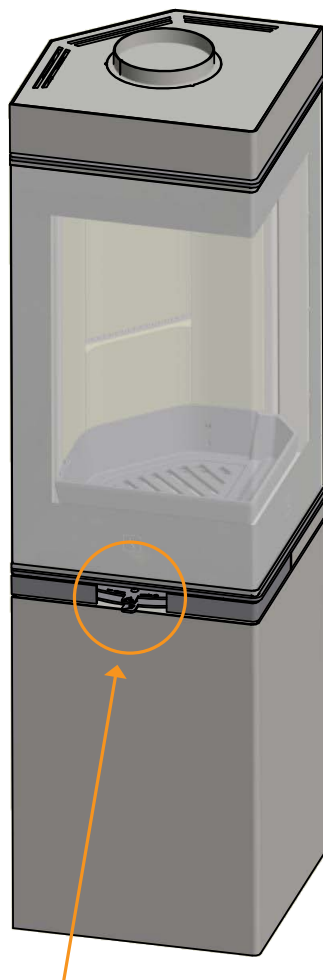
Dampers for primary- and secondary air
