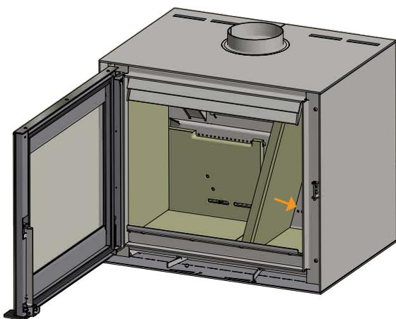
Mount the right rear plate. The rear burn chamber plates must be mounted so that the holes of the plates are placed precisely over the tertiary holes of the insert
