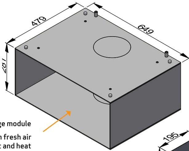
Large module with fresh air inlet and heat shield
