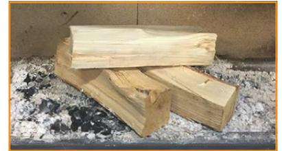
At the EN 13229-test the stove was fired as shown on the picture:
