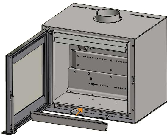
Place the bottom stones with the inclined edge turning to the rear and downwards
