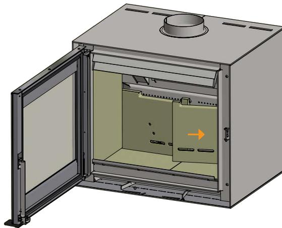
Mount the lower baffle plate. The baffle plate must be supported by the rear plates. Mount the pins and put the plate in place
